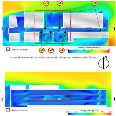
Streamline overlaid on Velocity Contour Map on the Longitudinal Section Plane
