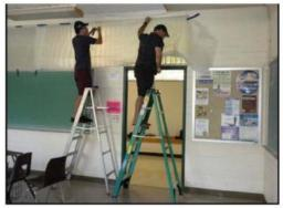
Installation of anemometers at the middle of the door ways
