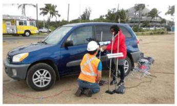
Installation of anemometers and pressure sensors
