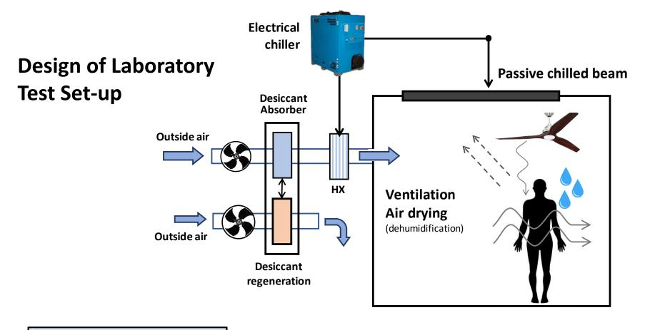
Latent heat removal = Dehumidification Advanced AC – Desiccant dehumidification & separate sensible cooling
