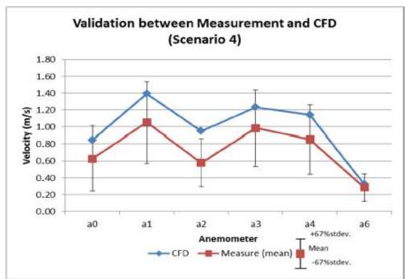
Comparison of air velocities between measurement and CFD for test scenario 4
