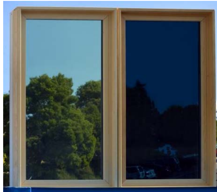
Prototype – Concept Window (Highly Insulating and Dynamic U Value 0.18 (SI U value 1.0) SHGC 0.04 – 0.34) Low cost unsealed center lite
