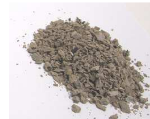
Before water-catalyzed self-degradation of cement at 200°C
