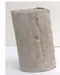
Before water-catalyzed self-degradation of cement at 200°C
