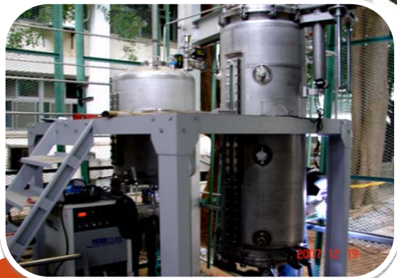
Biohydrogen production system
