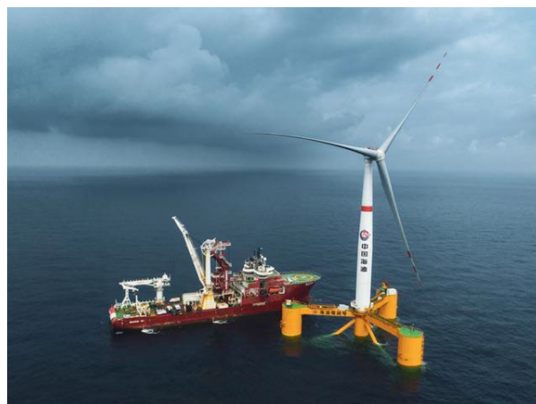
7.25MW漂浮式风电机组 7.25MW floating wind turbine
