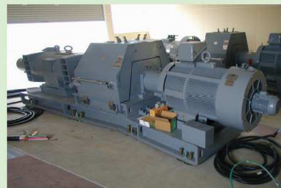
150kW rotating type generator (simulates WP, Co-generation)
