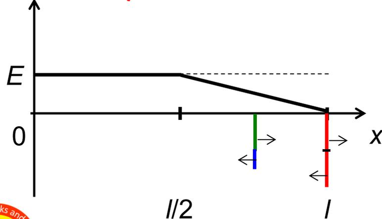
5. Back traveling wave is reflected with negative sign, then moving forward again
