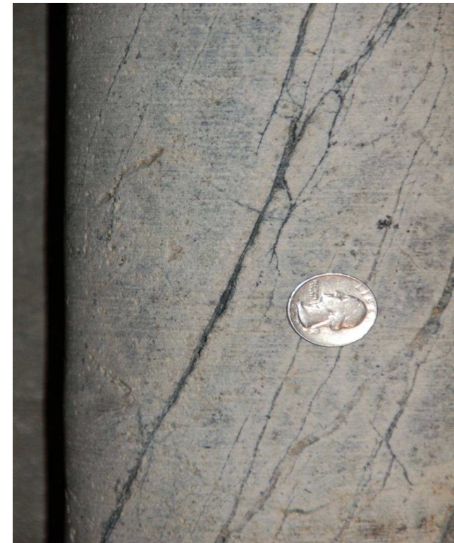
Fractured Geysers felsite: Fluid pressure lubricates small fractures like these, creating tiny induced seismic events detectable only to precision instruments
