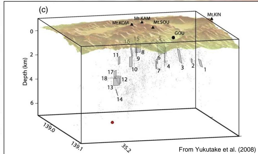
“Active seismic” (shot point) - “Passive seismic” (natural seismic signal) surveys - micro-earthquake surveys.
