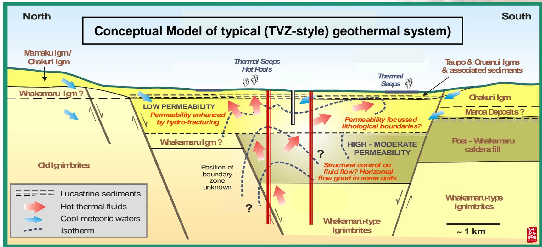
By **combining** geological, chemical and geophysical survey data, the geoscience team able to establish a conceptual hydrological model, which is updated through exploration and field development stages.
