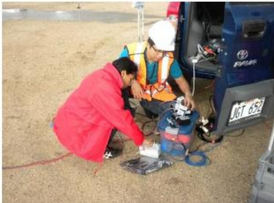
Installation of anemometers and pressure sensors
