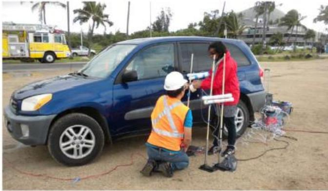
Installation of anemometers and pressure sensors
