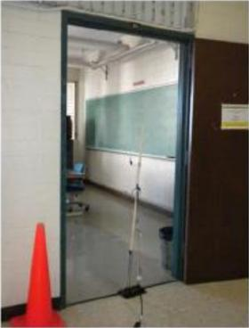
Installation of anemometers at the middle of the door ways
