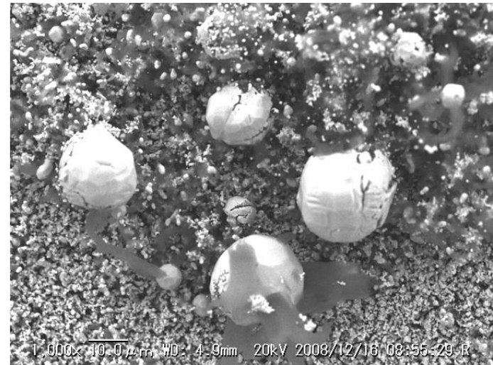
spent cell in test fueled by coal syngas
