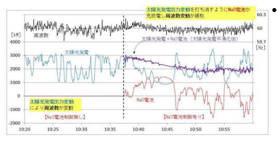
NAS Battery in Miyako Island Charge and discharge from Battery counteracts to output fluctuation from PV power generation
