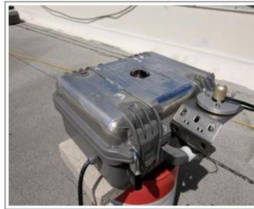
Upward looking sky imagers, supported with other instruments, are currently the best method to observe local cloud conditions at the time and space needed to predict short-term irradiance fluctuations
